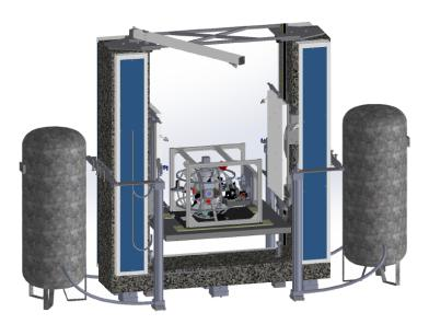
Figure 1: The science chamber situated on the Einstein elevator, which carries out a pre-programmed parabolic trajectory that yields up to 500 ms of weightlessness every 12 s. The platform and payload are guided by two vertically-mounted position-locked air skates, which produce low-friction motion with an excellent acceleration repeatability of 1 mg.
